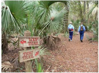
**Posting Height** – Hiking, off-road cycling and multipleuse marking should be four to six feet high on poles or posts along the trail, or five to six feet high on trees along the trail. Equestrian marking should be four to six feet high on poles or posts along the trail, or seven to eight feet high on trees along the trail.
